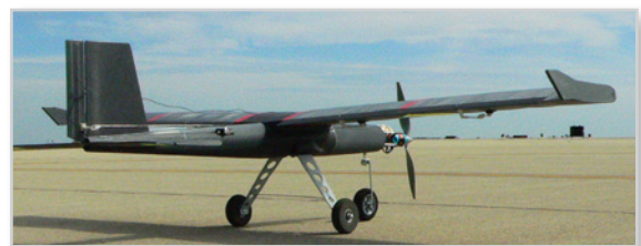
SelectTech Geospatial engineers perfected this drone through many iterations. Test flights were executed with functional prototypes made on an additive manufacturing system.
