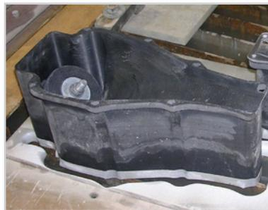
*Top NASCAR team, Joe Gibbs Racing, uses FDM to make fixtures, some of which have been in service for more than two years and have cut lead time and expense by an average of 70%.*
