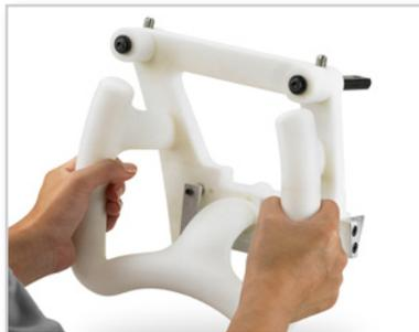
*Using FDM, BMW prints jigs and fixtures that would not be possible with conventional machining and fabrication. 3D printing allows them to be easier to use and more functional.*
