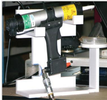
*When machined fixtures were quoted at \$12,000 and seven days, Thermal Dynamics opted to make them with FDM to save \$10,000 and several days.*
