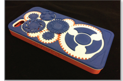
Figure 1: Multi-color FDM ABS-M30 mobile phone case.
