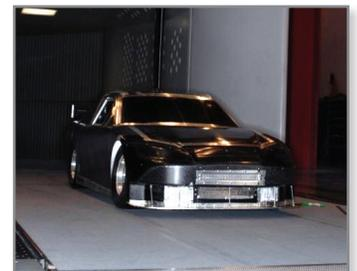
Figure 1: NASCAR teams rely on rolling-floor wind tunnels to analyze aerodynamics of their race cars.
