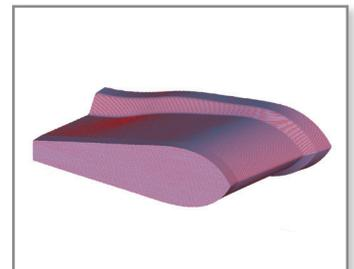
Figure 2: In this orientation, the airfoil's leading edge would have stepping that may alter wind tunnel results.
