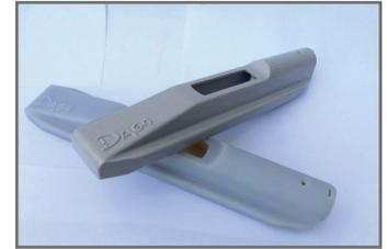
The PolyJet printed pattern (below) with the urethane cast part (top).
