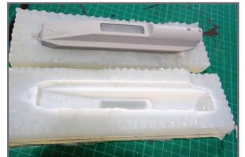
Silicone mold just after casting with the molding pattern.
