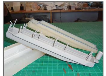
The urethane cast part with vents and runner next to the PolyJet master (top).
