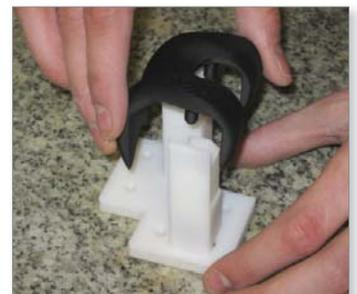
Figure 2: FDM contact elements designed to support an artificial knee.
