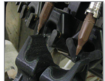
Numerous variations of this FDM part are needed by NTE’s customers for use in their daily operations.
