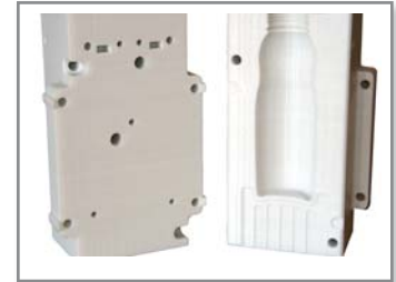
Figure 8: FDM blow molding tool made from polycarbonate.
