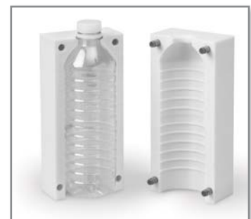
Figure 3: Blow mold constructed from the FDM process.
