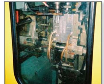
Figure 13: Prototype hybrid FDM tool mounted in blow molding machine.
