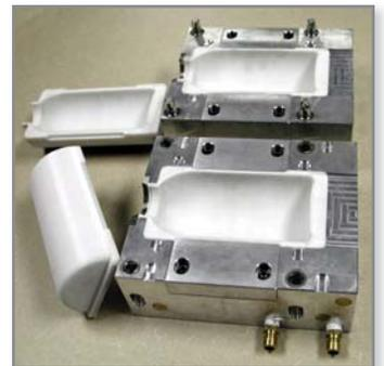
Figure 9: FDM hybrid tool with contoured inserts.
