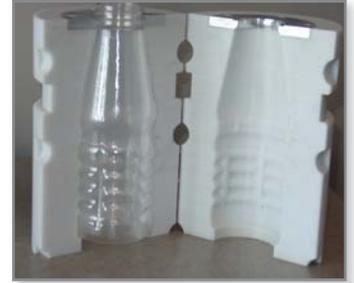
Figure 11: To mold the PET bottle, this hybrid insert uses a cylindrical design.
