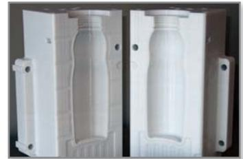
Figure 8: FDM blow molding tool made from polycarbonate.
