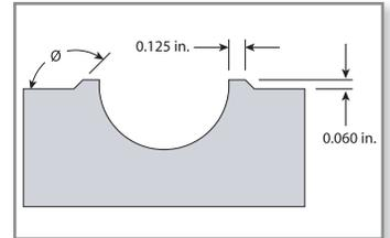
Figure 7: A rib is added to the tool design. The rib follows the contours of the mold cavity.
