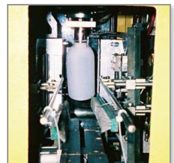
Figure 14: Prototype hybrid FDM tool opens and HDPE bottle is ejected.
