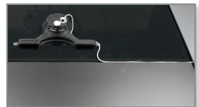
Figure 8: Remote camera mounted with neatly routed wires.
