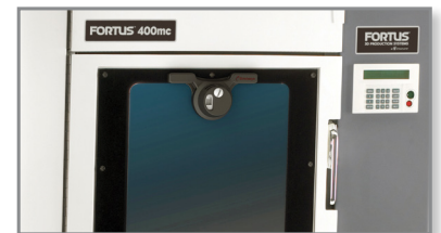
Figure 1: Remote camera system mounted on a Fortus 400mc ™ .
