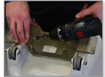
PolyJet drilling fixture with drill bushing used for accurate and repeatable hole placement.
