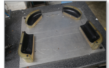
Wastebasket cover fixture that incorporates black soft-touch pads to protect surface finish of part.
