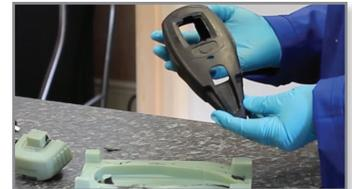
Figure 3: Removal of the boot from the mold.
