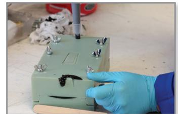
Figure 2: Injecting liquid silicone rubber into the PolyJet mold.
