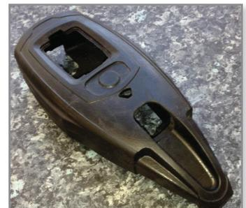
Figure 4: Functional prototype rubber boot produced with a PolyJet mold.
