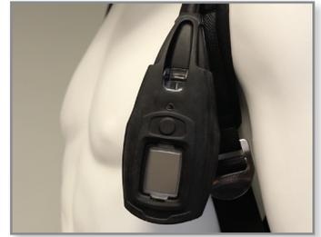
Figure 5: Mock-up installation of a DPG inside a rubber boot produced with a PolyJet mold.
