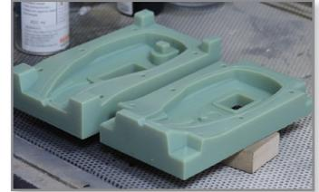
Figure 1: PolyJet Digital ABS<sup>™</sup> mold for a digital pressure gauge protective rubber boot.
