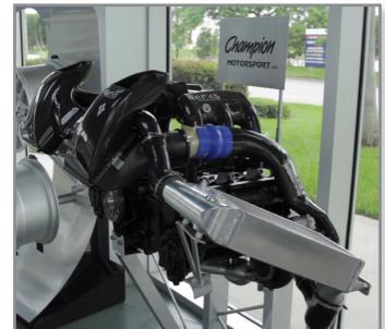
FDM soluble core-enabled components on a turbocharged engine.
