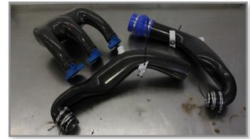
An array of complex, composite ducts made using FDM soluble cores.
