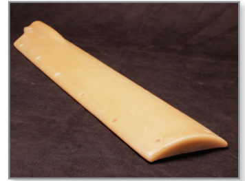
Cast urethane distal cover ready to be finished, painted and mounted on the MRI coil assembly.
