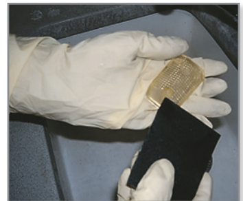
Figure 3. Dry-sanding the part. Sand all surfaces to smooth the model.
