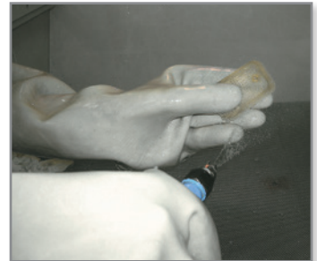
Figure 2. Wash model. Pressure wash the model to remove all support material.
