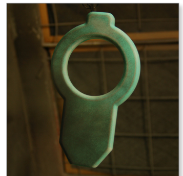
Applying a second coat of primer.
