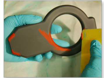
Using body filler to touch up the part.
