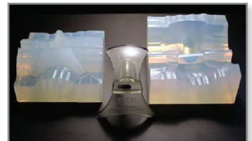
Inkjet master model and silicone mold
