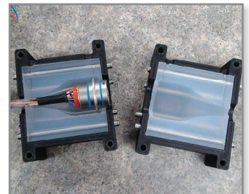
RTV silicone mold, made with an FDM master, for overmolding operation
