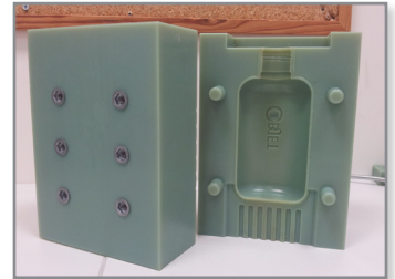
This inkjet 3D printed mold has metal thread inserts to ensure the best assembly on blow-molding machine platens.
