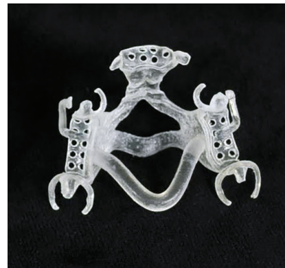
This cast frames, top, was created with the help of 3D printed bio-compatible (MED610) material, bottom.
