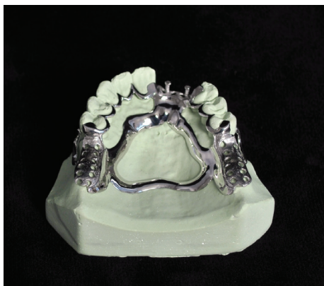
Partial frames, like these two maxillary (upper) arches, can be time- and labor-intensive if created via traditional manufacturing. Digital dentistry improves the time to make and accuracy of partial frames.
