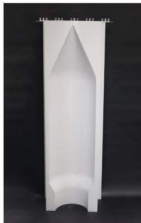
2. Stratasys Infinite-Build 3D Demonstrator part – rocket-fairing tool
