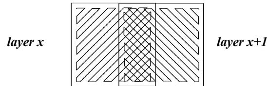
Figure 2: Raster Fill with Raster Direction at  $90^\circ$  to one another
