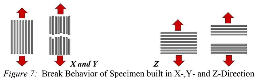
Figure 7: Break Behavior of Specimen built in X-, Y- and Z-Direction
