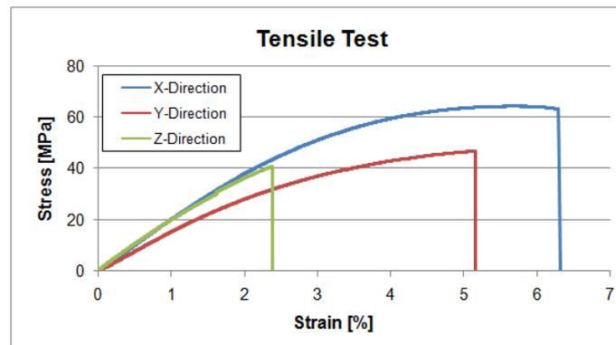
Figure 5: Compare of Stress-Strain Curves from different Build Directions
