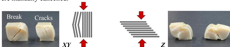
Figure 10: Break Behavior of Specimen built in XY- and Z-Direction
