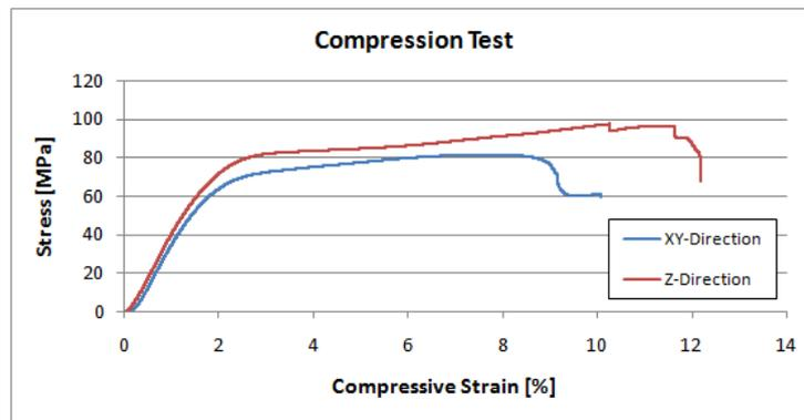
Figure 9: Compare of Stress-Strain Curves from different Build Directions
