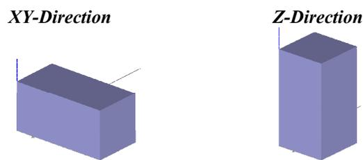
Figure 8: Build Direction of Specimen for Compression Test (XY and Z)
