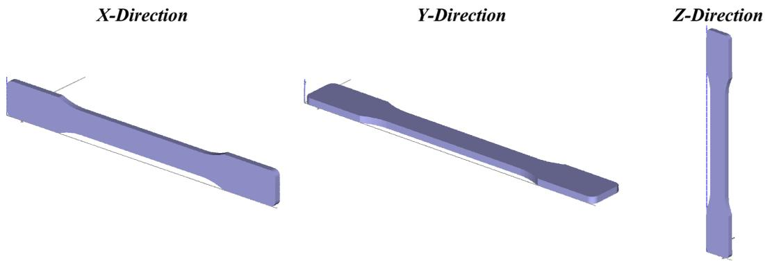
Figure 3: Build Direction of Specimen for Tensile Test (X, Y and Z)
