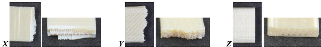
Figure 6: Fractures of Specimen built in X-, Y-, and Z-Direction
