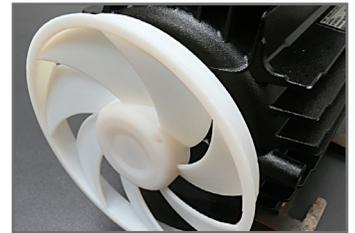
*3D printed fan on engine axis for testing.*
