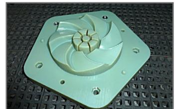
*Core side of 3D printed mold.*
