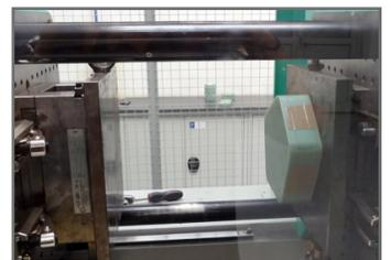
*3D printed mold mounted on the injection molding machine.*
