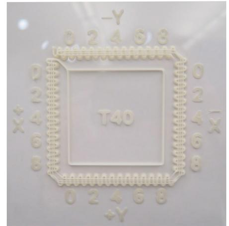
Figure 8: New T40A tip calibration box.
