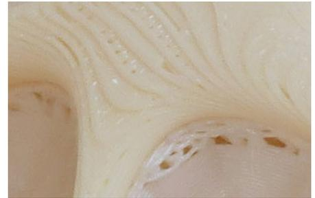
Figure 4: Default stair stepping of layers.
