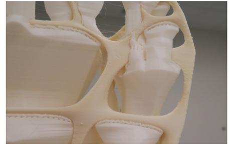
Figure 2: A part with small, complex toolpaths.
