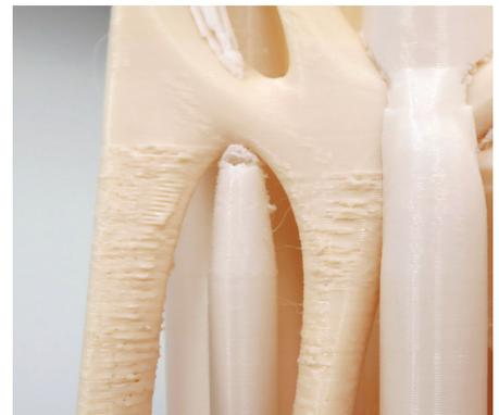
Figure 6: Deformation due to instability.
