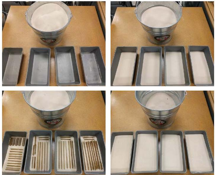
Figure 2 - Specimens should be placed in a sand bath to prevent deformation while being annealed.
