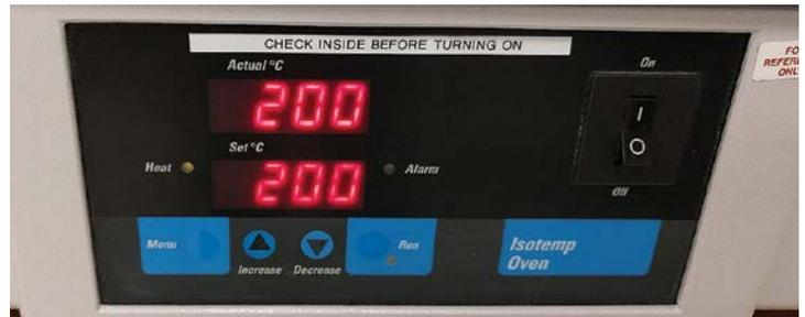
Figure 1 - Annealing can be completed in standard industrial ovens.
