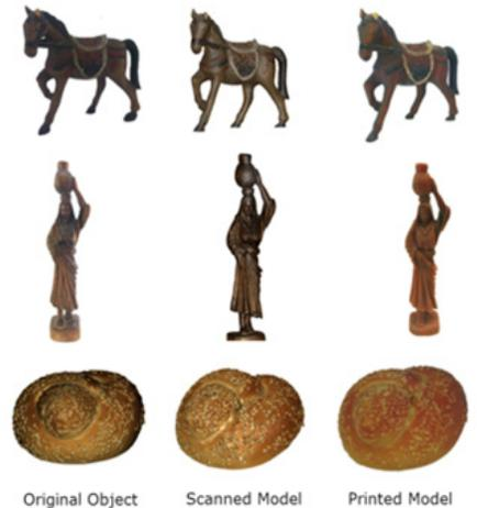
Figure 4: Scanned color models and the printed result.
