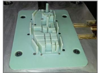
Core mold insert assembled to the mold base.
