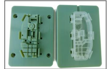
Part produced with a PolyJet mold that is ready for functional testing.
