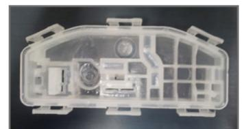
Seuffer’s polyethylene housing created with a PolyJet tool.
