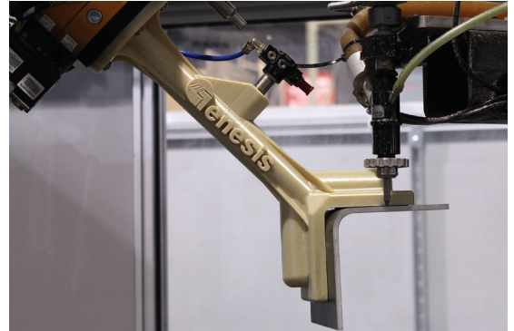
Figure 4: FDM EOAT gripper used in a waterjet operation.
