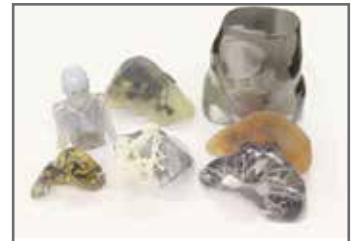
The multi-material capabilities of the Objet500 Connex3 is crucial for displaying interior elements of body parts.
