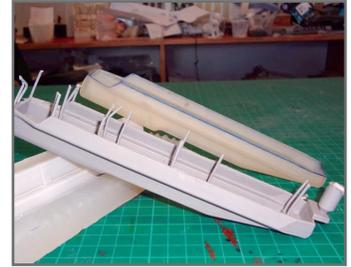
The urethane cast part with vents and runner next to the PolyJet master (top).
