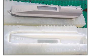
The silicone mold just after casting with the molding pattern.
