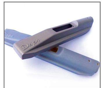
*The 3D printed pattern (below) with the urethane cast part (top).*
