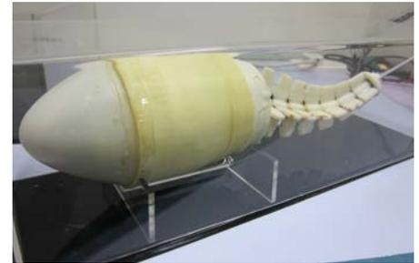
The fish-shaped model to be used underwater as an assessment instrument.
