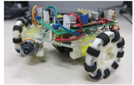
A multi-directional car with wheels 3D printed on a Fortus 3D Production System
