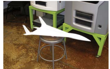
Embry-Riddle Aeronautical University students use Dimension 3D Printers to build scale models for wind tunnel testing, like this model aircraft.
