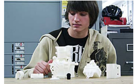
Silverman reverse engineered Briggs & Stratton small engine parts and printed physical models on their Stratasys 3D Printer.
