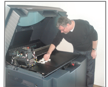
The company uses the Objet Eden500V to makes customized veneer trial models
