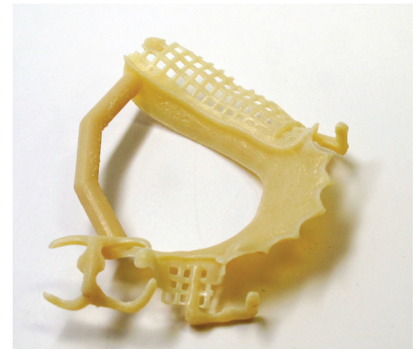
A removable partial framework model 3D printed in MED620 material.
