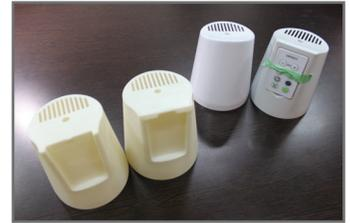
3D printed prototypes of the fan next to their finished counterparts.
