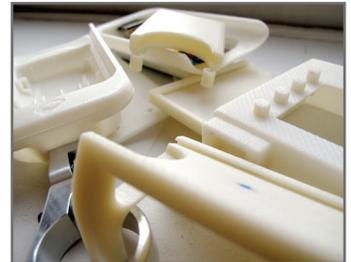
*Pedal Brain printed early prototypes of these different devices with uPrint.*
