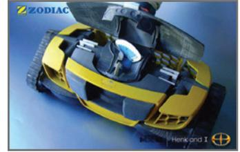
Zodiac's MX 8 pool cleaner works on a motor that has few moving parts, reducing potential failure. Working FDM prototypes (above and bottom) helped design firm Henk and I develop the motor iteratively.
