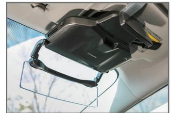
3D printed prototypes helped validate designs to steady the projector and fit perfectly.
