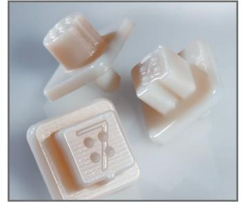
*The high accuracy of the Objet 3D Printer has greatly improved production of tactile-realistic models that visually impaired people can test.*
