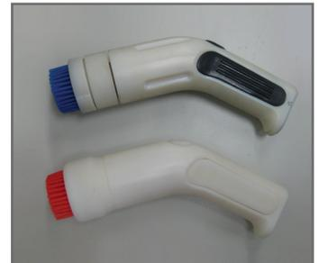
3M Korea selected PolyJet™ technology to produce prototypes with multiple materials.
