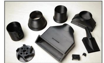
*RedDOT 3D printed these durable nylon prototypes in-house with FDM.*
