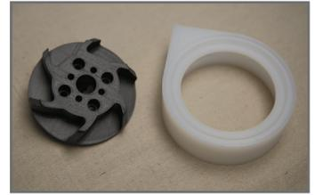
*The 3D printed impeller prototype (black) works with its PC mate to push an ice slurry through a chilling system.*
