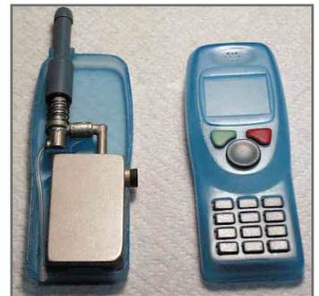
*This Super Soaker, disguised as a cell phone for sneak attacks, was modeled using FDM.*
