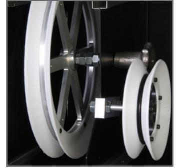
*The pull-force test fixture uses the wheel on the left to give the material filament the proper radius.*
