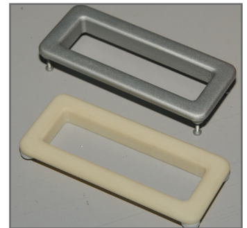
Top: Painted FDM oil level indicator frame. Bottom: FDM oil level indicator before painting.
