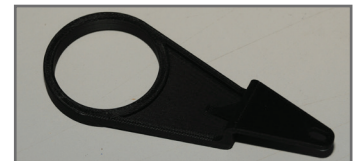
This drive piece was produced on a Fortus machine to be installed directly into a press system as an end-use part.
