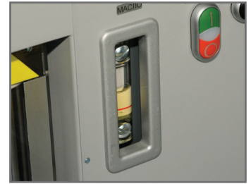
The frame to house the oil level indicator on the hydraulic laboratory press was produced with ABS plastic on a Fortus machine.
