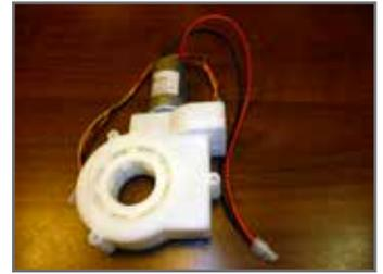
*The complicated motor assembly for the head swinging mechanism was built out of ABS too.*
