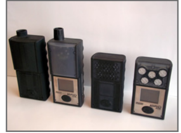
Industrial Scientific Corporation's MX6 gas detector is a lifesaver for miners and utility workers worldwide. Engineers use the Dimension 3D Printer to make full-scale prototypes for testing, ensuring a user-friendly finished product.
