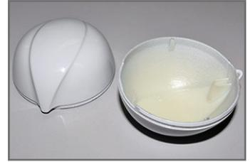
*Shower head prototypes made easy with PolyJet 3D Printing technology.*
