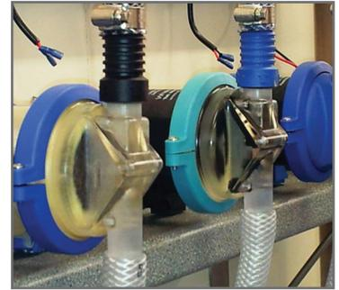
Functional testing of diaphragm prototypes that were created with 3D printed injection molds.
