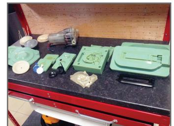
3D printed injection molds for various applications made with ABS material.
