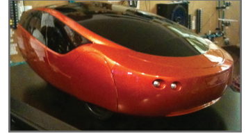
The Urbee is the first prototype car ever to have its entire body 3D printed with an additive process. It was created using Dimension 3D Printers and Fortus 3D Production Systems at RedEye On Demand.
