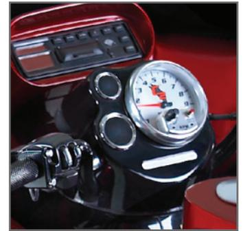
Painted polycarbonate gauge pod installed directly on the bike.
